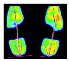
The D30 Insole (left) reduces the pressure felt on the underside of the foot (green = low pressure). The competitor insole (right) fails to match this (red = high pressure). The acceleration control is also maintained much better by the D30 Insole, highlighted by the fact that the black dotted line is more consistent along the pink midline.\*
